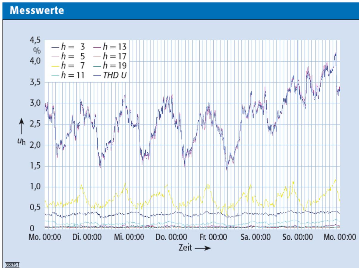
Fig. 1: Distortion in the supply voltage from a public 20-kV network (measured values)
