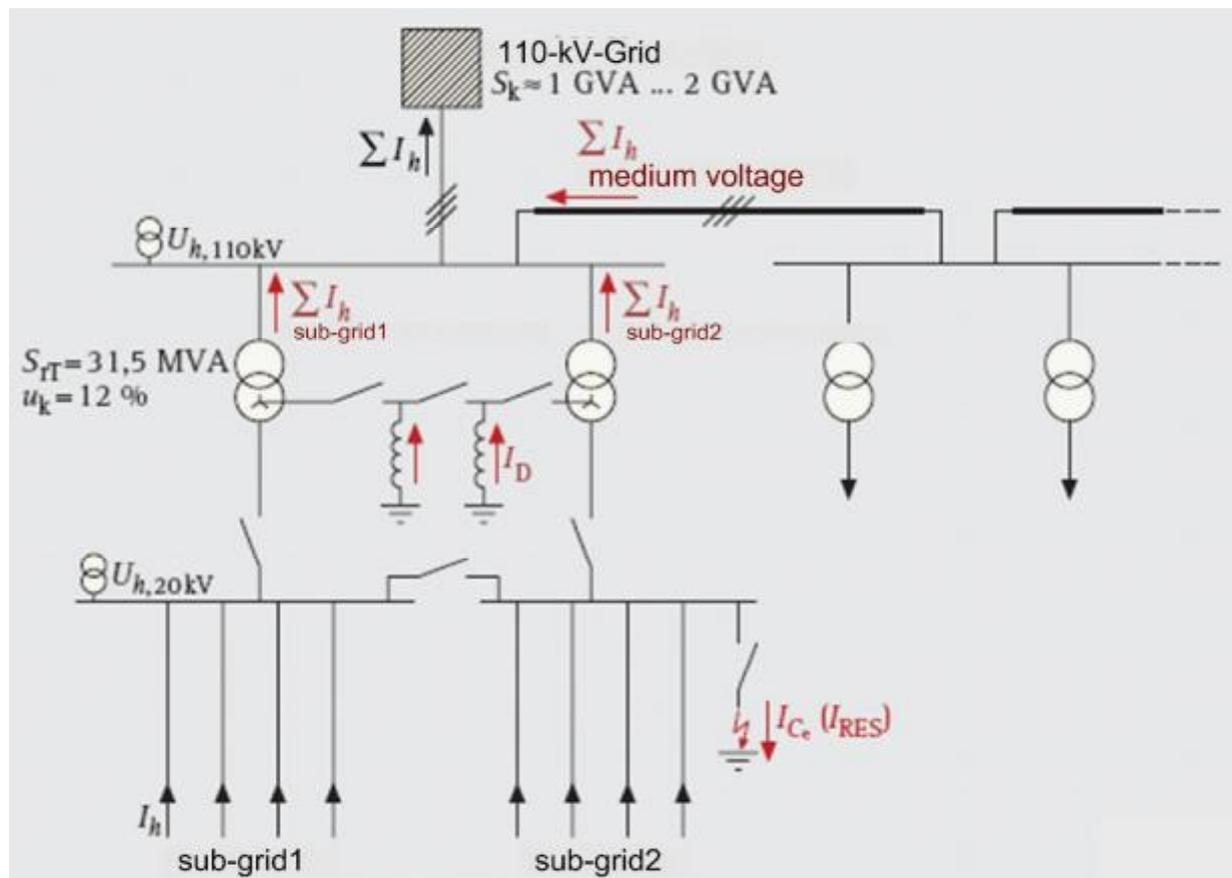
Fig. 2: Simplified basic structure of the MV network
