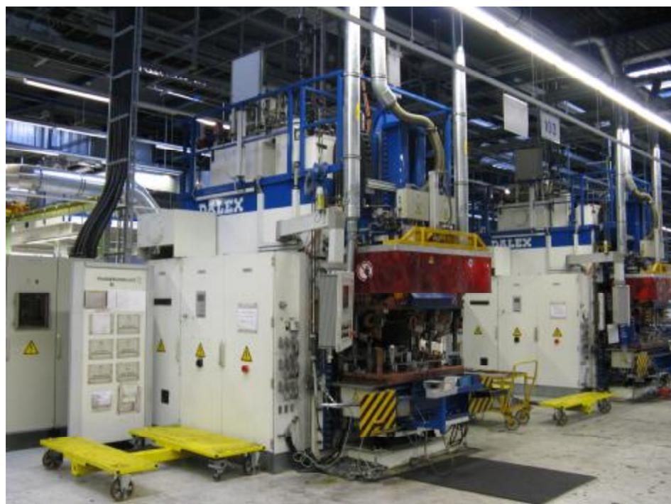
Fig 1. Electrical pressure welding machine in automotive manufacture
