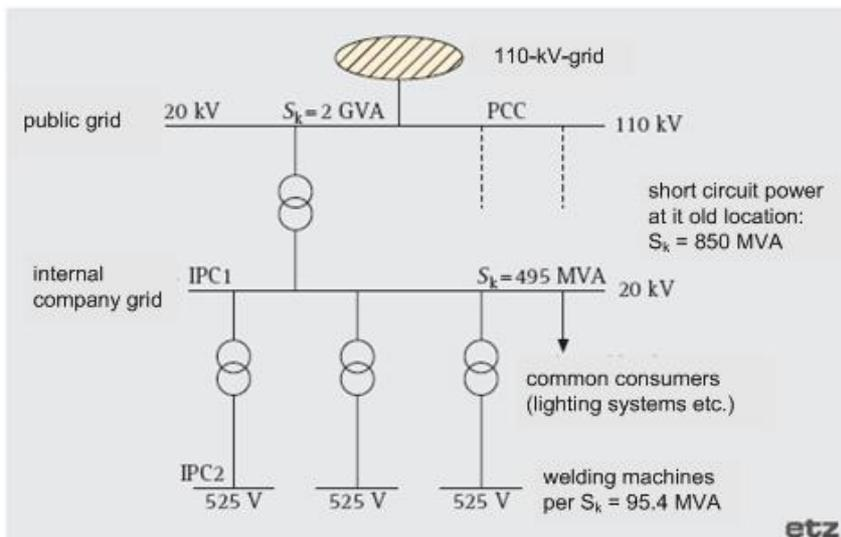
**Fig. 4: Highly simplified grid diagram for the network supplying power to the welding machines**
