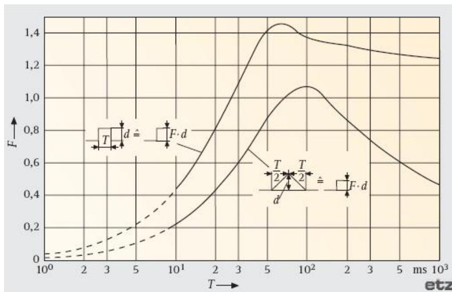
Fig. 2: Form factors for rectangular pulses [2]
