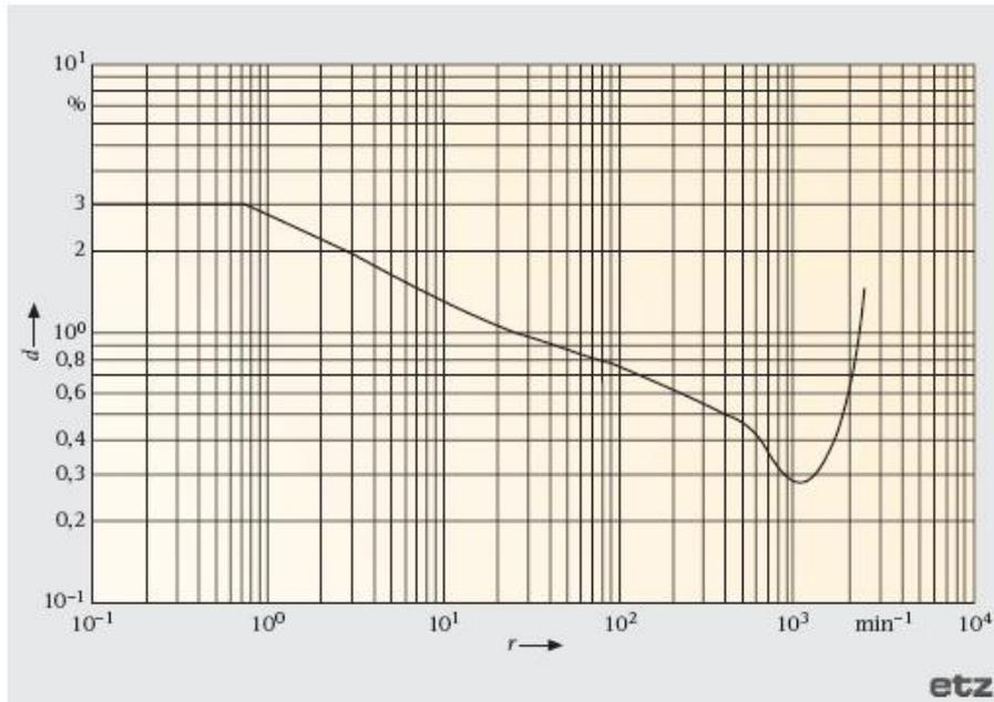
**Fig. 1: Reference curve  $d_{\text{ref}}(r)$  for  $P_{\text{ref}} = 1$  and regular, rectangular voltage changes [1]**
